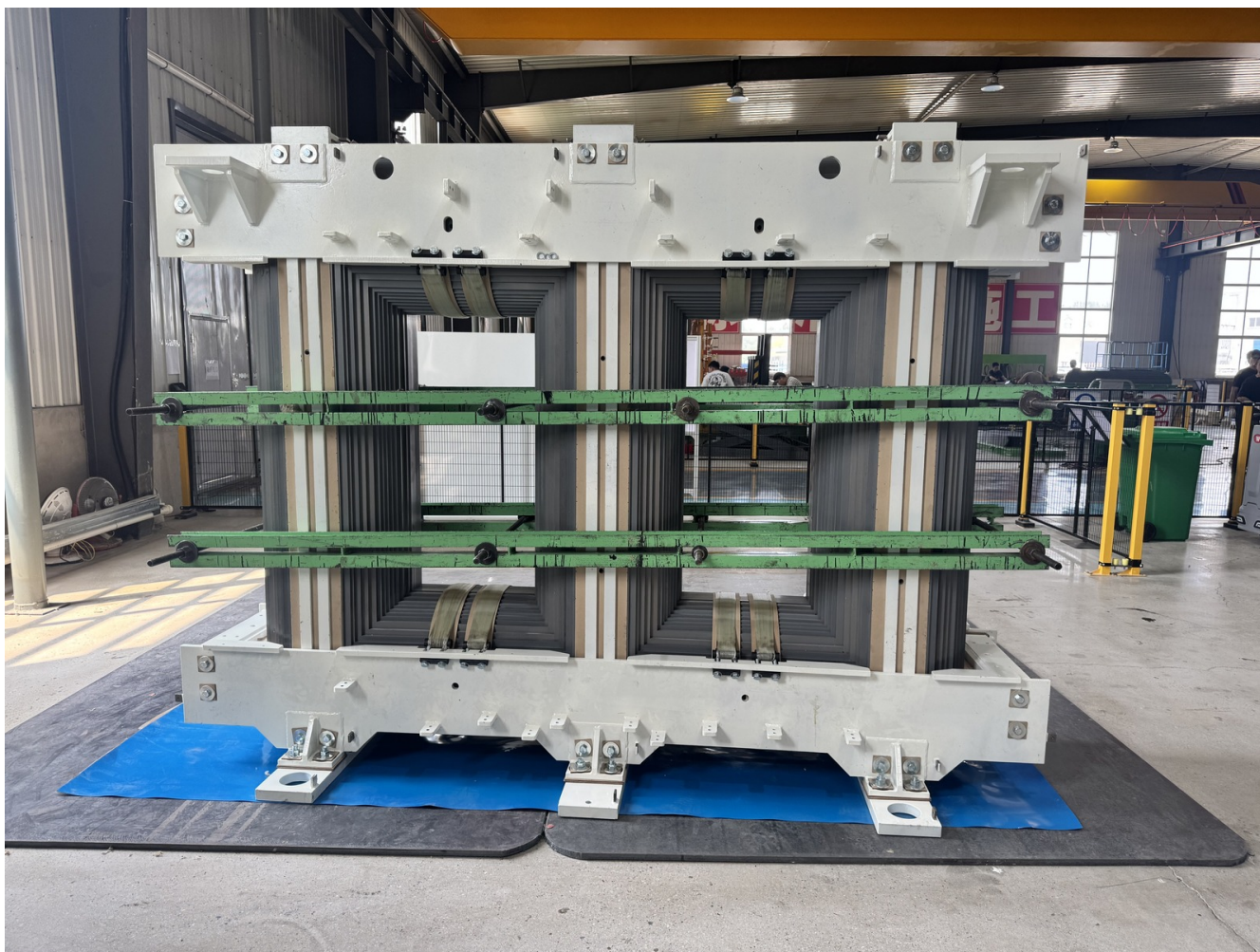
Assembled transformer core manufactured by Chenfan Electric.
